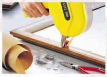
Save time and effort for double matting, filleting, dust covers, and more – With **Scotch® ATG 700** or **ATG 714 Applicators** and **Scotch® ATG Tapes**, a touch of your finger applies a precise strip of adhesive at the same time as the liner rewinds into the applicator.
