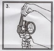
3. Pull tape over smoothing roller allowing roll to rotate freely off tape wheel. To increase or decrease unwind tension see diagram 2 above.
