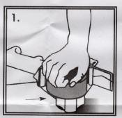
face. Push roll of tape onto Be sure tape unwind orientation has sticky side down (per diagram 1 above).
