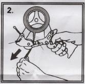
1. Place dispenser on flat sur- 2. Pull 5-6 inches of tape off and thread (sticky side down) tape wheel until fully mounted. between smoothing roller and metal loading gate.
