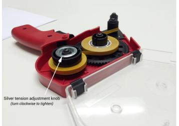
Another photo showing more of the release liner on the take up spool sitting at the same level as the roll on the main spool. If the tension on the gun is set too low the liner will also not be wound correctly on the take up spool.
