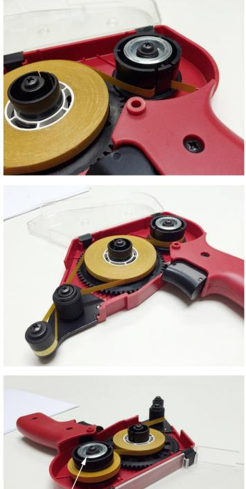
When the release liner on the take up spool as shown to the left. Make sure no adhesive is left on the release liner being fed into the take up spool (it is applied at the far left roller and none should be left on the release liner at this point).
