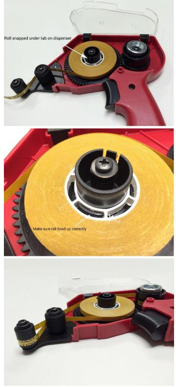
When inserting the roll into the gun make sure it snaps down underneath the tab which helps to hold it in place. Also wind it clockwise as shown in the photo to the left.
