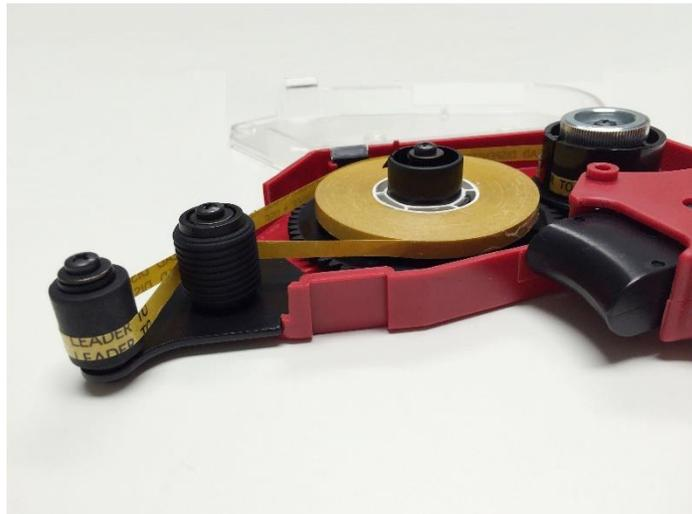
When winding the tape into the gun make sure to wind enough into the gun so that you are at least past the part of the roll with the written "USE LEADER..." instructions since the adhesive will not start until after that part.
