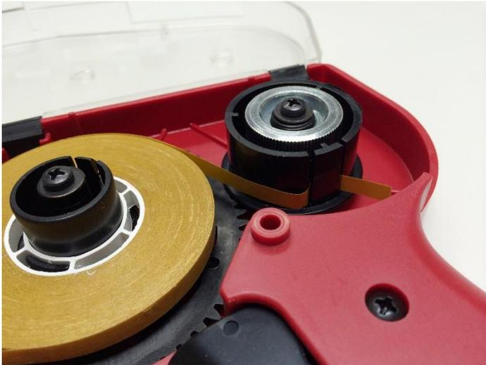
When the release liner on the take up spool as shown to the left. Make sure no adhesive is left on the release liner being fed into the take up spool (it is applied at the far left roller and none should be left on the release liner at this point).
