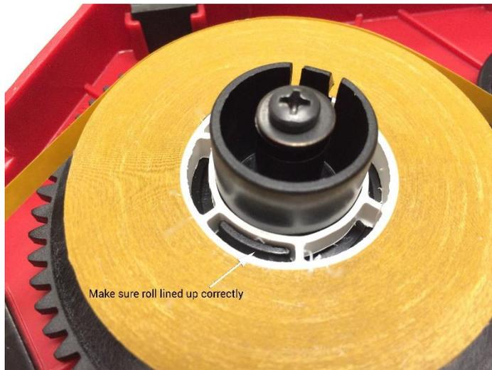
Also make sure the roll is lined up correctly and is seated with the lower tab sitting within the core section as shown in the photo to the left.
