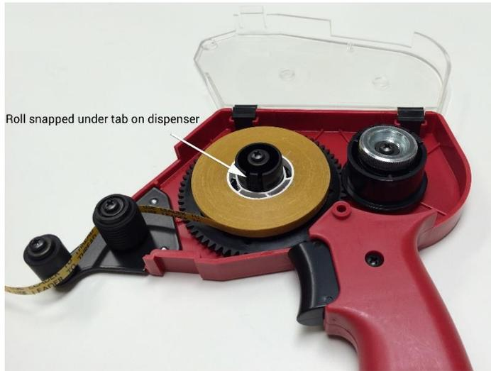
When inserting the roll into the gun make sure it snaps down underneath the tab which helps to hold it in place. Also wind it clockwise as shown in the photo to the left.
