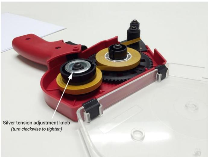
Another photo showing more of the release liner on the take up spool sitting at the same level as the roll on the main spool. If the tension on the gun is set too low the liner will also not be wound correctly on the take up spool.
