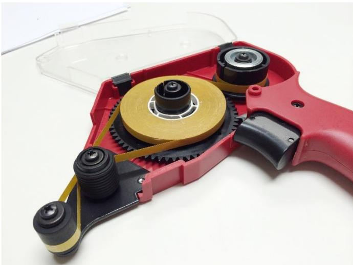
Make sure as the release liner is being wrapped around the take up spool it is on the same level as the main spool. You don't want the release liner to break or be telescoped upward on the take up spool which happens if the gun's tension is set too high.
